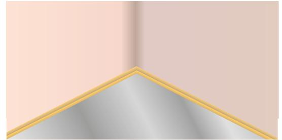
2. Fix a 25mm batten around the perimeter of the room.
