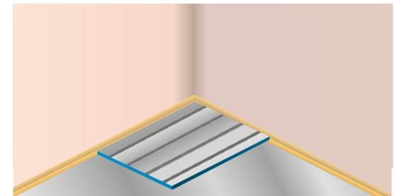
4. Start to lay the pipework into the preformed Foil Board using the HydroHeat CAD Design. Each insulation board will have pre-formed bend to allow for the return pipework.
