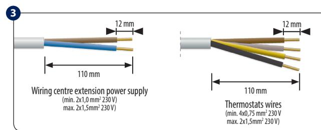
Remove the appropriate piece of insulation from the wires.
