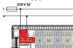
Power supply for wiring centre is 230 V ~ 50Hz.
