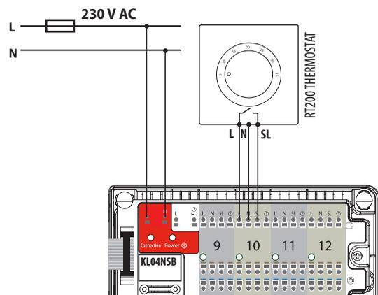
• Connecting ON/OFF battery-powered thermostat with voltage-free COM / NO output contacts (e.g. 091FL, RT310, RT510)
