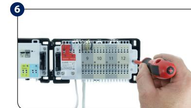
Adjust the wires and screw the main housing of the wiring centre extension to the rear housing.
