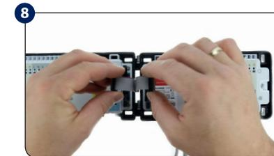
Connect the serial cable to the KL08NSB and KL04NSB connector.
